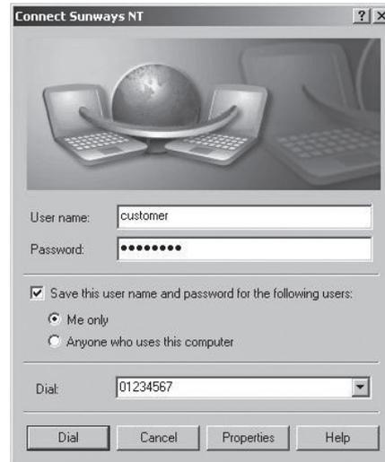
13. Click «Dial» to establish the connection. After the connection is established you can start the Sunways Browser by entering the IP address of the Solar Inverter in the address line of your web browser.
