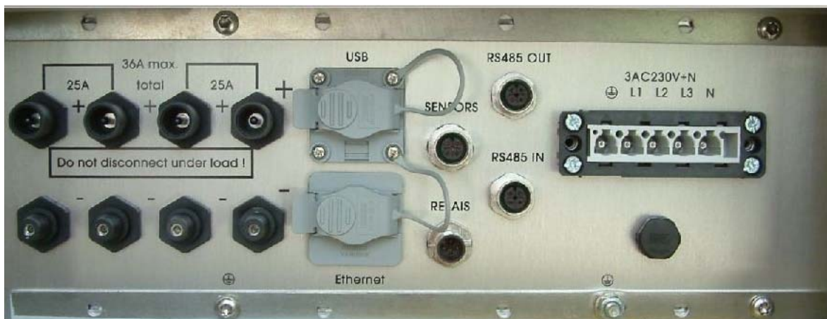
Figure No.7 Connection of device
