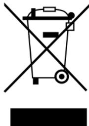
Dispose of the packaging and replaced parts according to the rules applicable in the country where the inverter is installed. Do not dispose of the inverter with normal domestic waste. The inverter conforms to RoHS. That means that the device can be taken to municipal disposal sites for household appliances. AE takes the inverter back completely. Please contact the Service team!
